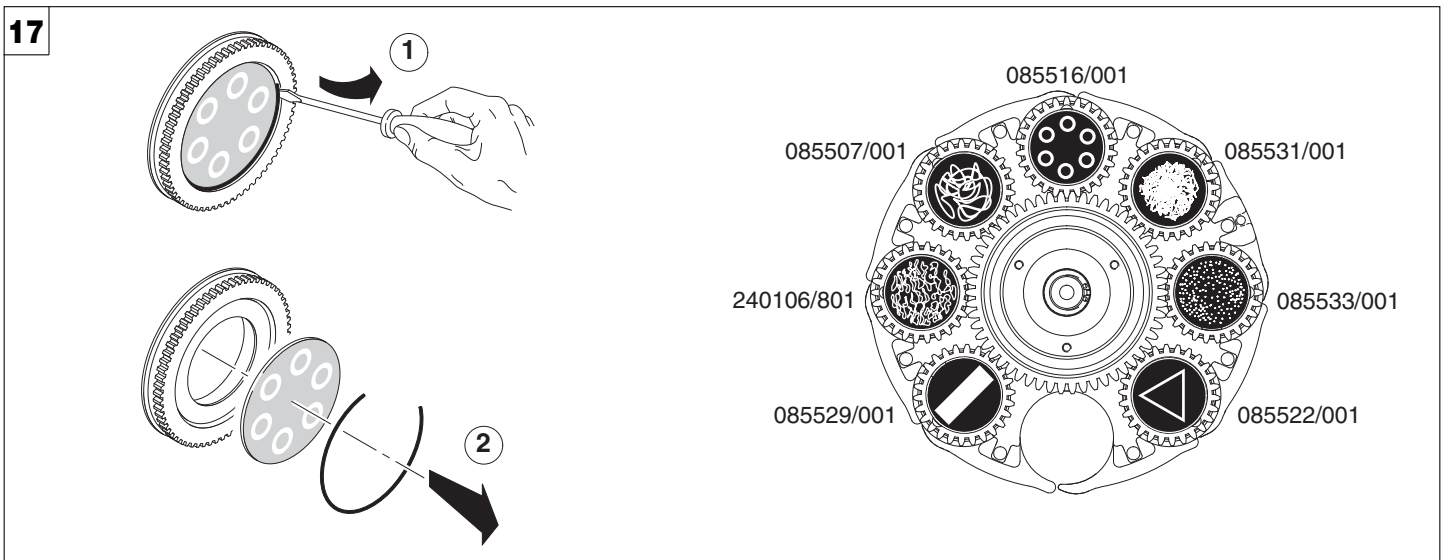
Replacing rotating gobos (ø 25.7 mm - max 23 mm image – thickness max 1.1 mm) - Fig. 17
